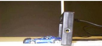
This car is too close the photogate. The "flag" of the second car should trigger the photogate immediately after the collision.
